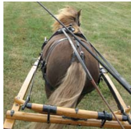
Shaft is too narrow
